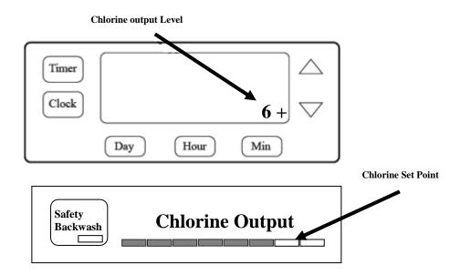
Your Filtrite salt chlorinator will always attempt to adjust the output so that the actual output level matches set point level. At times when the chlorine output level is lower than the set point, check the salt level in your swimming pool at your local Clark Rubber. Alternatively, you may have a low voltage supply to the chlorinator (less than 240Volts) or the water may be colder than usual.
